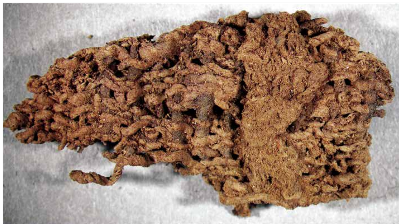
Figure V.2. Layers of four different unbalanced, plain-weave fabrics. Photo: Margaret Ordoñez.
