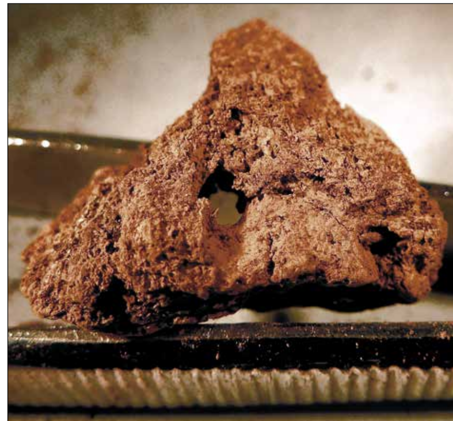
Figure V.3. Degraded fabric with penetrating holes possibly caused by sewing threads. Photo: Margaret Ordoñez.
