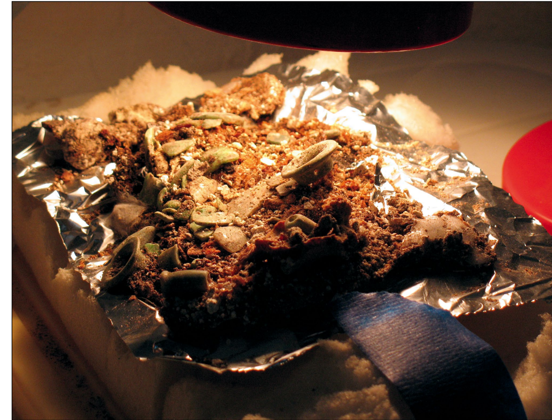
Figure III.3. Complex items from Burial 9 were block-lifted using cyclododecane wax, later sublimed beneath incandescent light in the laboratory. Photo: Catherine Magee.
