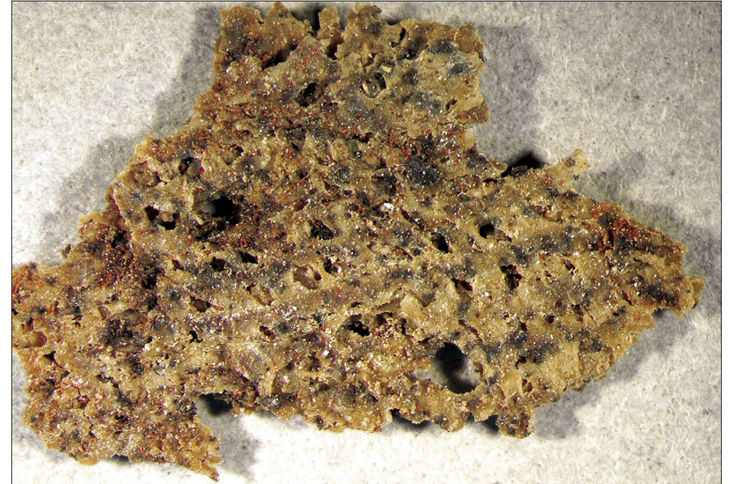
Figure V.10. Degraded barkcloth with characteristic spacing of fibrous components. Photo: Margaret Ordoñez.
