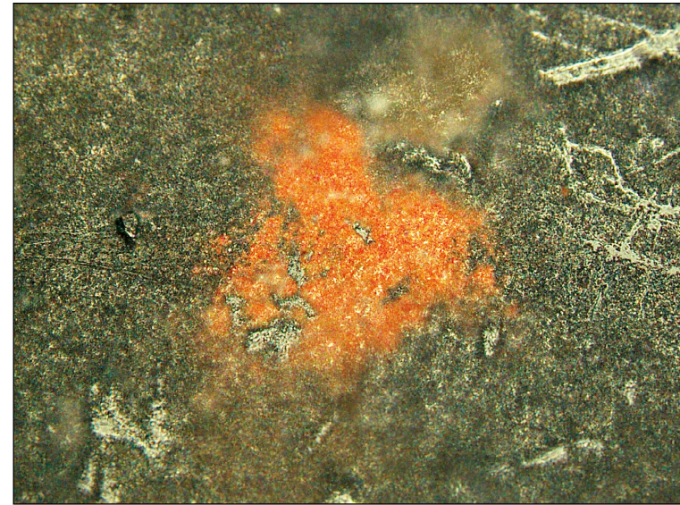
Figure II.4. Red residue on the macroblade (200x). Photo: Kazuo Aoyama.
